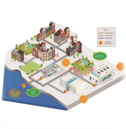
District heating & cooling networks powered by innovative CO2 loop technology
